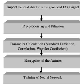
Fig. 4. Algorithm for Classification of Neural Network.
